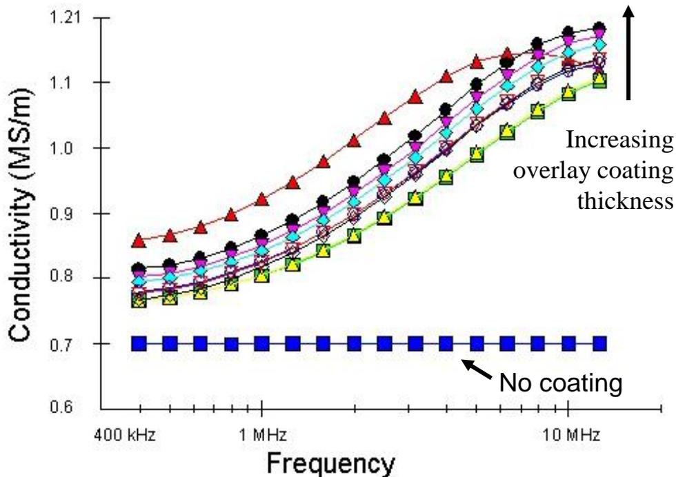
Note that the results are essentially not affected by increasing lift-off, i.e., by adding a 25- $\mu\text{m}$  thick shim between the sensor and part.
